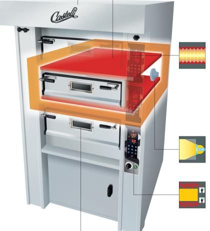
Electric resistance units are made of an alloy of nickel and chromium and are set on proper frames situated beneath the plane and along the ceiling of the baking boxes. This particular setting guarantees a more uniform heat diffusion, together with a more effectiveness in the cooking process and the capability of maintaining the temperature.
