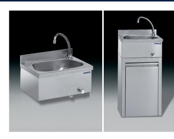
95 models. Soundproof basins, 2 depthts 60 and 70 cm. Jointed sinks and rounded edges, splash guard upstand, overflow pipe and extractable perforated false bottom. Models on legs, on side panels and with doors. Accurate finishing: no sheetmetals with sharp edges. Sturdy structure made entirely of stainless steel AISI 304 Cr.Ni. 18/10.
